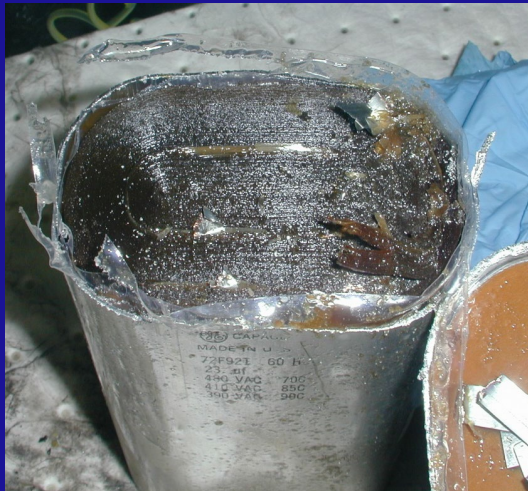
Cobra style street light capacitor with oil-impregnated paper
